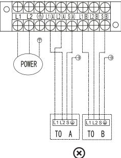
**NOTE:** If the client wants to perform the wiring himself, refer to the following figures. Run the main power cord through the lower line-outlet of the cord clamp.
