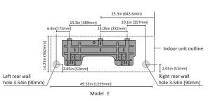
**NOTE:** When the gas side connective pipe is  $\Phi$ 5/8in(16mm) or more, the wall hole should be 3.54in(90mm).
