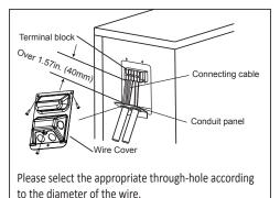
Outdoor Unit Wiring Diagram is located on the inside of the wire cover on the outdoor unit.
